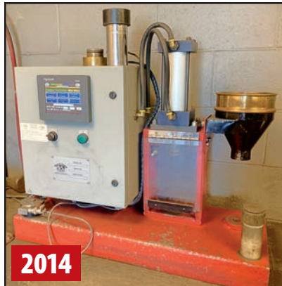
2014 GREEN SAND CONTROLS PME-ACTS PRECISION TEST STATION
